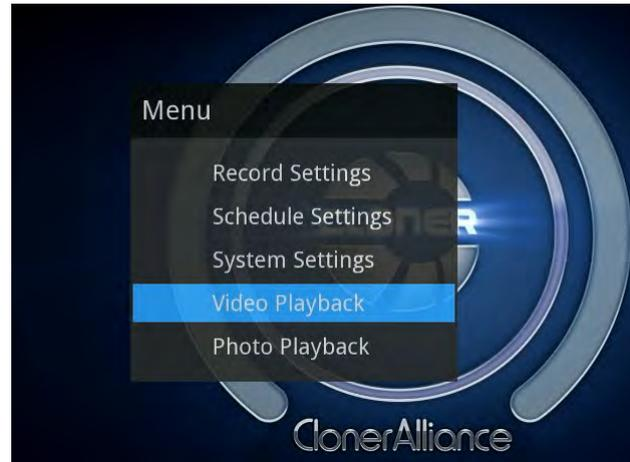
Choose the file you want to play back by using the four arrow buttons on the remote control, and press PLAYBACK button on remote to start/pause playback. You also can enter fullscreen by pressing OK button on the remote control.
