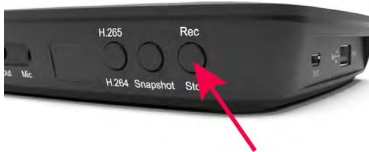
4. Press the Rec/Stop button again on ClonerAlliance UHD Pro, then the LED will blink blue/green alternately, which indicates the recorded video is being saved.
