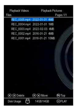
3. Select your desired file by using the up and down arrow buttons on the remote control/ViewPro. And then press OK to playback the selected video in full screen.
