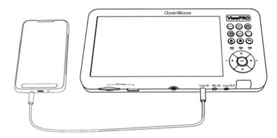
After connected audio device to "Line in", it will directly mix audio to HDMI embedded audio. It also can be monitored from "Line out" and output devices.
