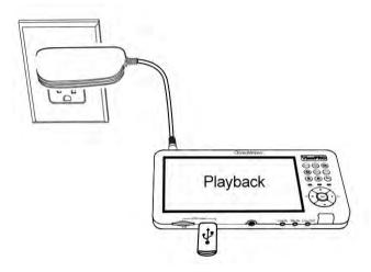
1. After inserted the storage device to ClonerAlliance ViewPro and powered it up, please press the "PLAYBACK" button on ViewPro or on the remote control to enter the playback mode. You will see a prompt "Select storage device".
